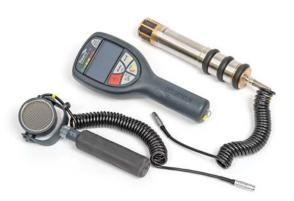
An intrinsically safe, weatherproof monitor with dual probe capability - the ultimate tool for obtaining accurate NORM Measurements in hazardous areas or difficult conditions.
